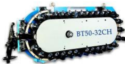
Figure 2.2. Typical CNC tool magazine (Source: ATC Machining Co., 2006)
