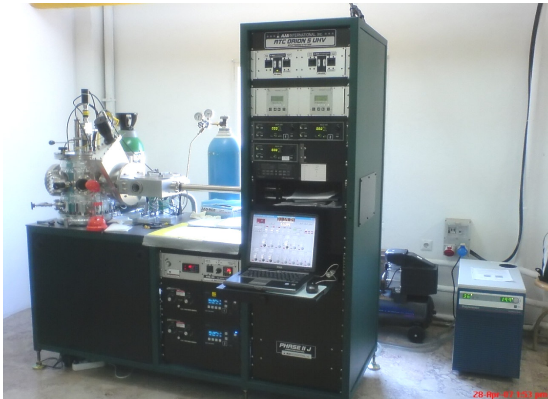
Figure 3.2. ATC Orion 5 UHV Sputtering System (AJA International) in the Department of Physics at Izmir Institute of Technology.
