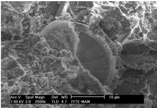
Figure 3.9. SEM images of diatoms embedded in calcite crystals in grey limestone.
