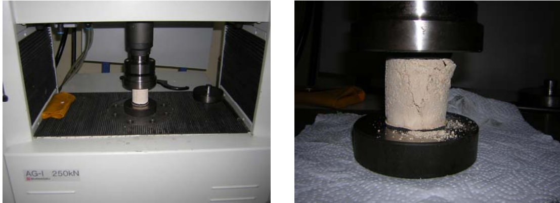
Figure 3.37. Uniaxial compressive strengths and modulus of elasticities of test mortars.
