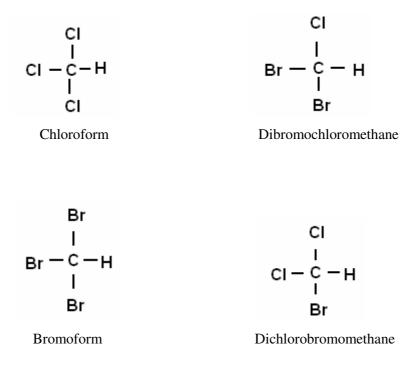
Figure 2.2. Molecular structure of THMs
