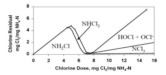
Figure 2.1. Theoretical breakpoint curve (Source: USEPA 1999)
