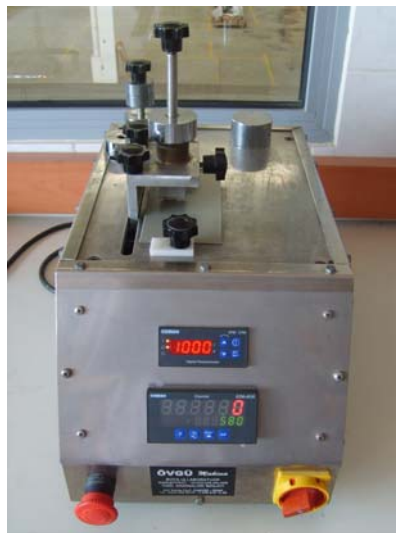
Figure 3.8. MEK Double-Rub Tester
