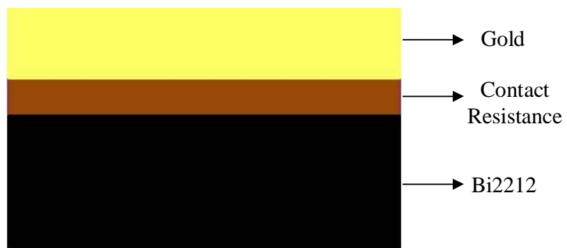
Figure 4.4. Side view of mesa to show the contact surface resistance between gold layer and surface of Bi2212
