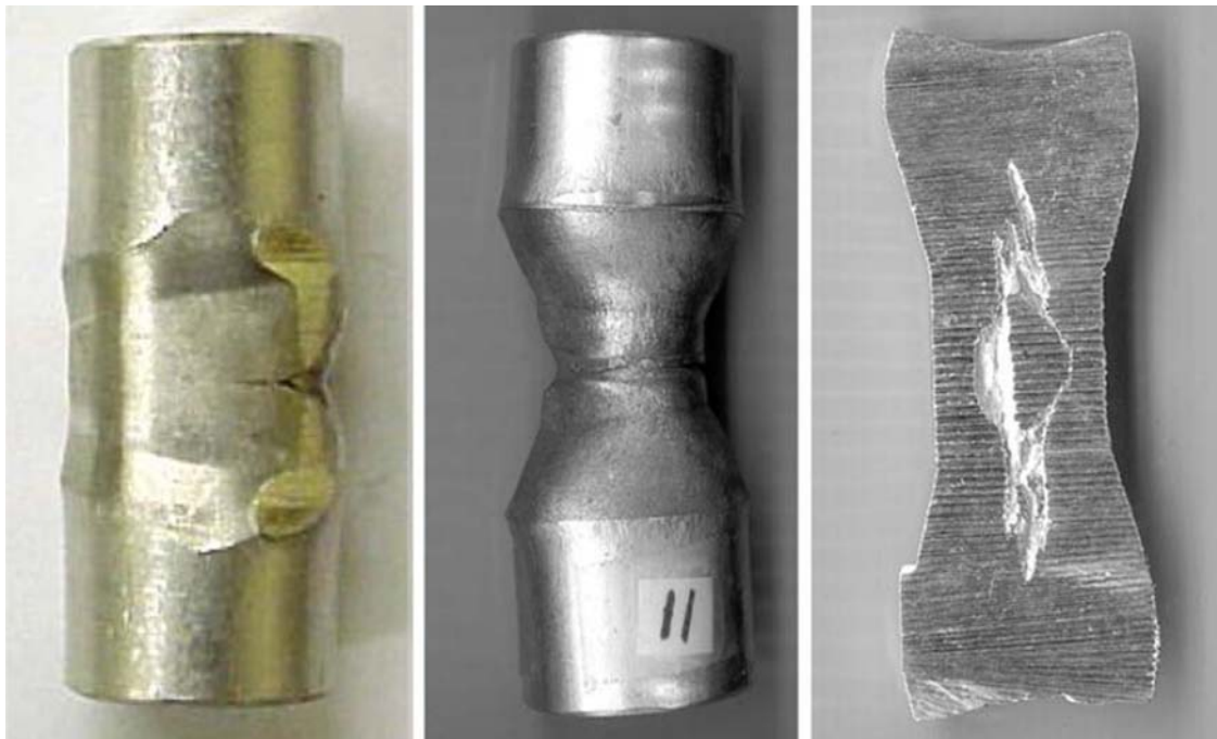
(a) Excess slip (b) surface defect (necking) (c) Internal void
