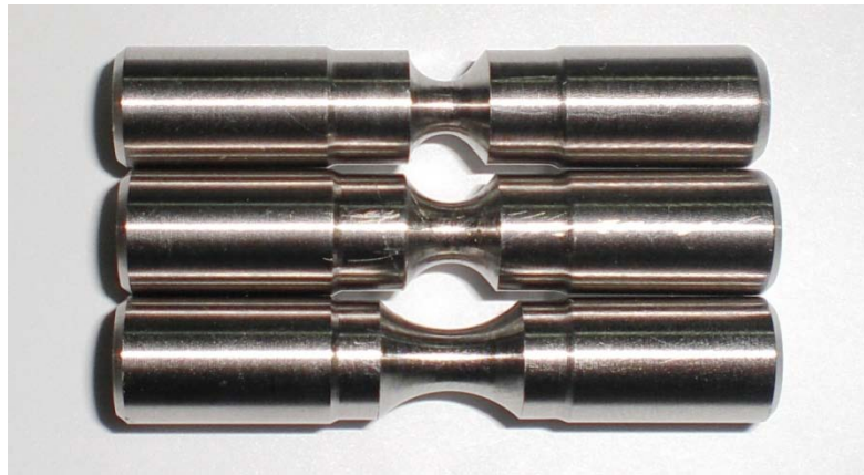
Figure 3.3. Static notch Ti6Al4V samples of R=2, 3 and 6 mm.
