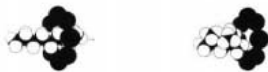
Figure 3.4. Illustrations of molecular sieve effect. Straight chain molecule of normal octane (left) passes through an eight-ring zeolite; branched molecule of iso-octane (right) cannot (Falnigen. 1991).
