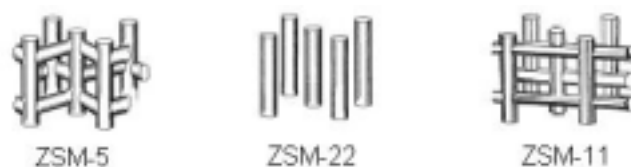
Figure 2.3. Illustrations of three-dimensional pore structures of ZSM-5, ZSM-22 and ZSM-11.
