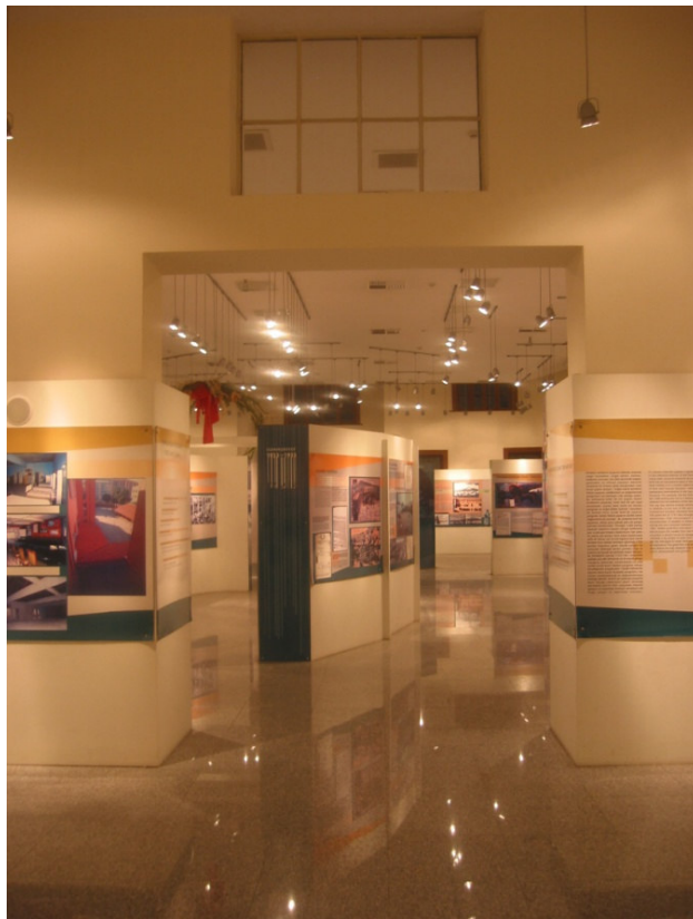
Figure 4.27. Reflected glare from floor under halogen spotlighting
