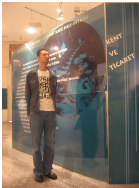
Figure 4.29. Reflected glare on vertical panels under halogen spotlighting. Both the light sources and the standing person are reflected on the surface.
