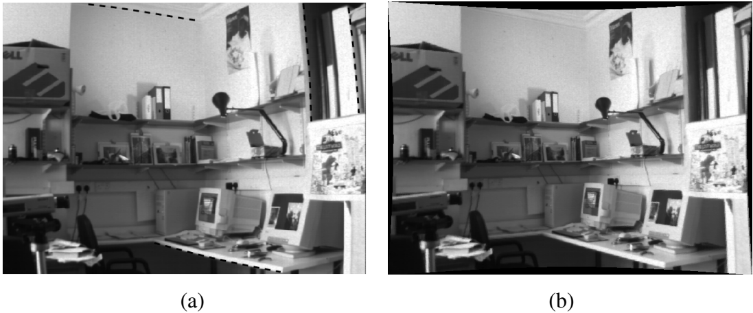
Figure 2.8. (a) An image before undistort process (b) after undistort process.
