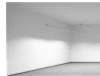
Figure 2.4. Direct, diffuse lighting
