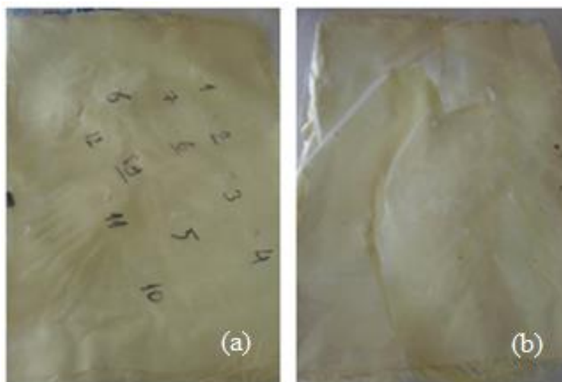
Figure 5.53. Images after ballistic test of 15 layers of neat aramids from (a) front and (b) back side
