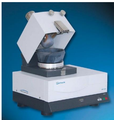
Figure 4.4. Automatic agate mortar used for grinding dried particles
