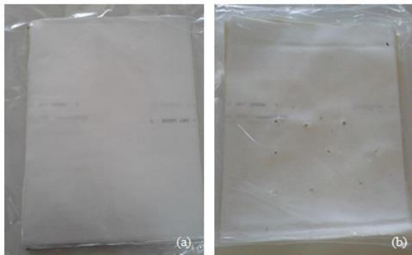
Figure 5.58. Images of STF/UHMWPE fabric composite containing STF prepared with 30 wt. % fumed silica and 70 wt. % PEG 300 from front side (a) before and (b) after ballistic test
