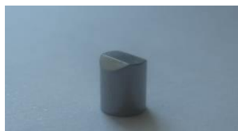
Figure 4.17. 1.1 \pm 0.03 gram (17 grain ) fragment-simulating projectile
