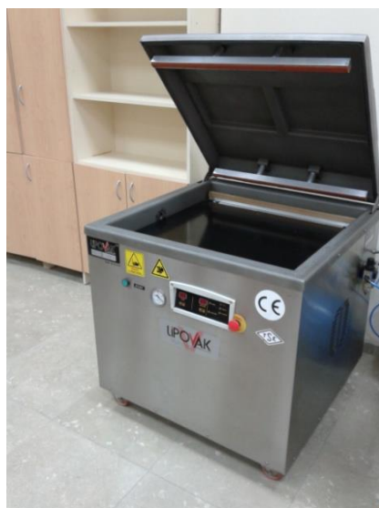
Figure 4.9. Packing machine used for STF/aramid composite packaging.
