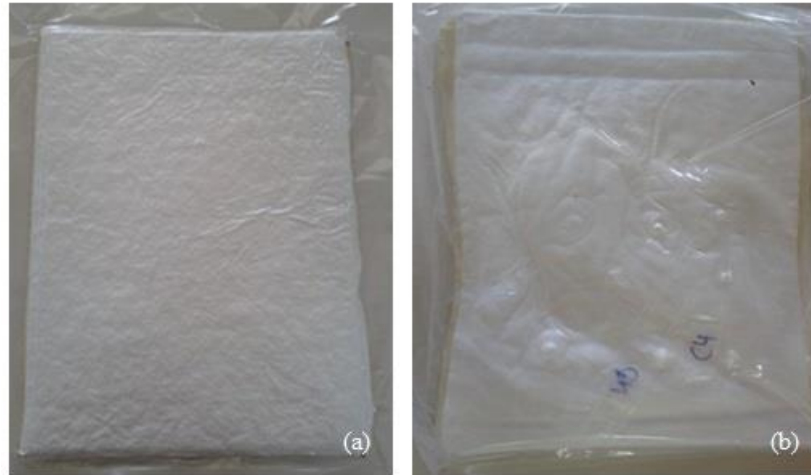
Figure 5.59. Images of STF/UHMWPE fabric composite containing STF prepared with 30 wt. % fumed silica and 70 wt. % PEG 300 from back side (a) before and (b) after ballistic test
