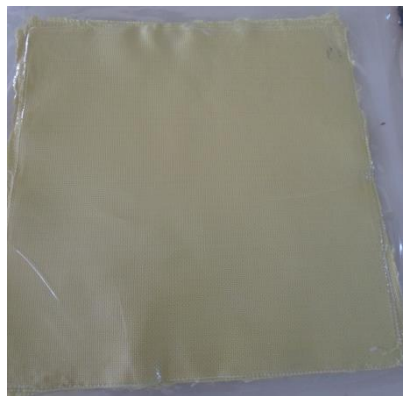
Figure 5.50. Front image of neat fabric before ballistic test
