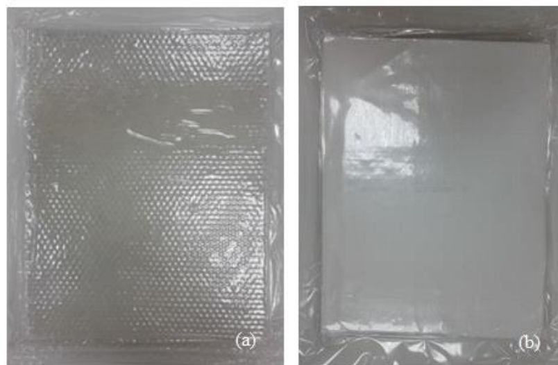
Figure 5.60. Images of STF/PP honeycomb composite containing STF prepared with 30 wt. % fumed silica and 70 wt. % PEG 300 (a) front and (b) back side
