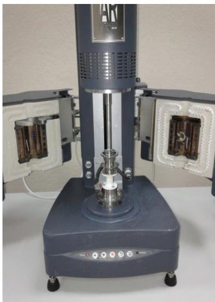
Figure 4.10. TA Instruments AR2000ex oscillatory rheometer used within the experiments
