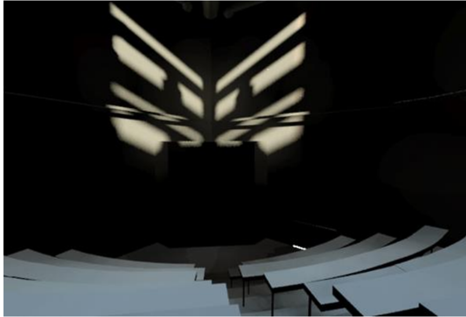
Figure 28. Daylight incidence on the whiteboard / projection screen by 3ds Max Daylight Analysis Tool (March 21, 15:30)
