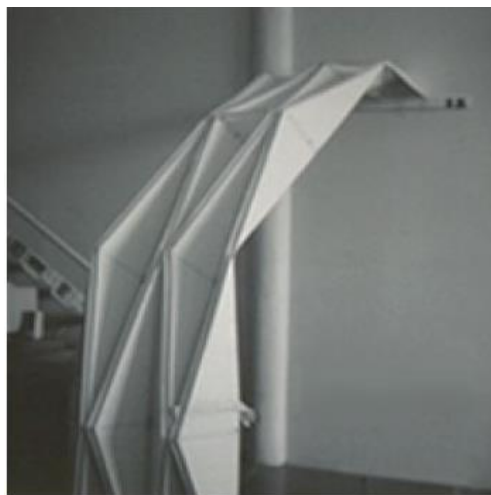
Figure 3.23. Half-shell with 3 Triangulated panels by “Kinetic Design Group” (Source: Fox & Yeh, 1999)
