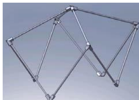
Figure 5.11. A product design of the foldable shelter frame (Source: Chen, 2003)
