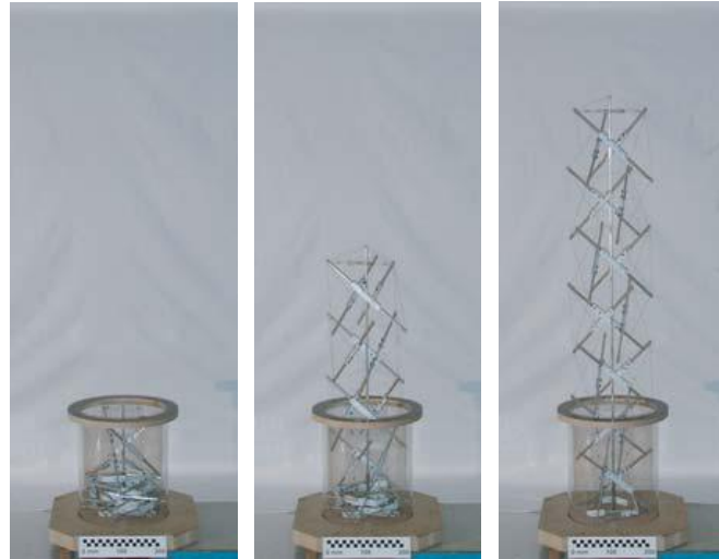
Figure 3- 41 Physical model of Pellegrino's folding mast at different stages of folding process (Source: Tibert & Pellegrino, 2003)
