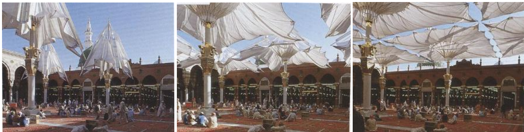
Figure 3- 53 Umbrellas in Madinat during opening process (Source: Otto & Rasch, 1995)
