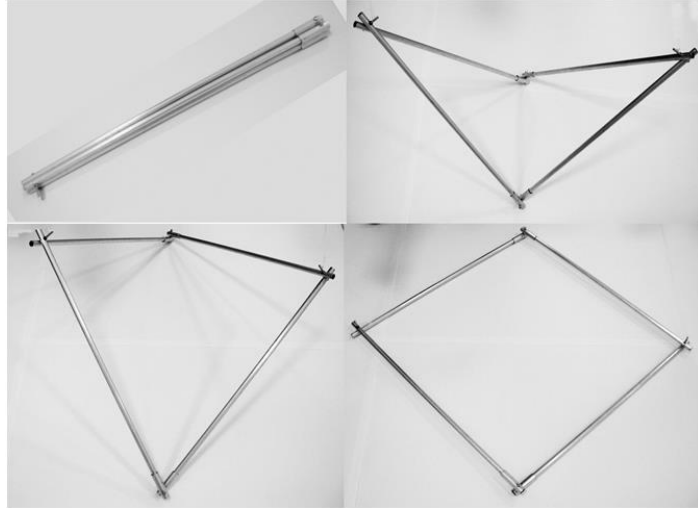
Figure 5.18. Transformation capacity of the proposed novel mechanism (Korkmaz, Susam & Akgün, 2013)
