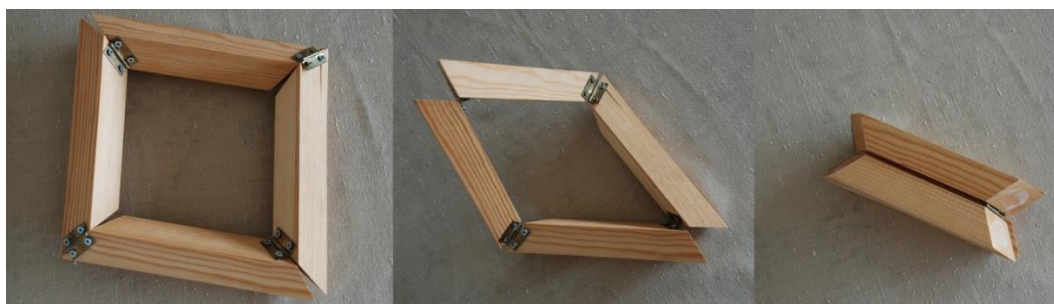
Figure 5.13. Bennett linkage with skew square cross-section bars
