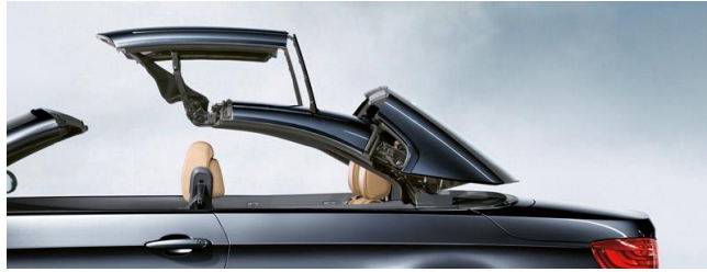
Figure 3.49. Retractable hardtop of the car; is an example for structural mechanisms (Source: Bmw, 2013)
