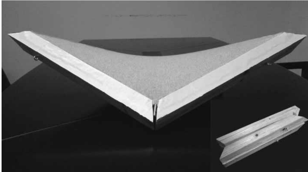
Figure 5.15. A deployable membrane structure in the folded and unfolded configurations (Source: Yu, Luo, & Li, 2007)
