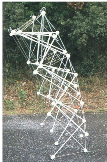
Figure 3- 42 René Motro's prototype of a double-layer, double-curvature tensegrity system, continuous cables join the nodes (Source: Robbin, 1996)
