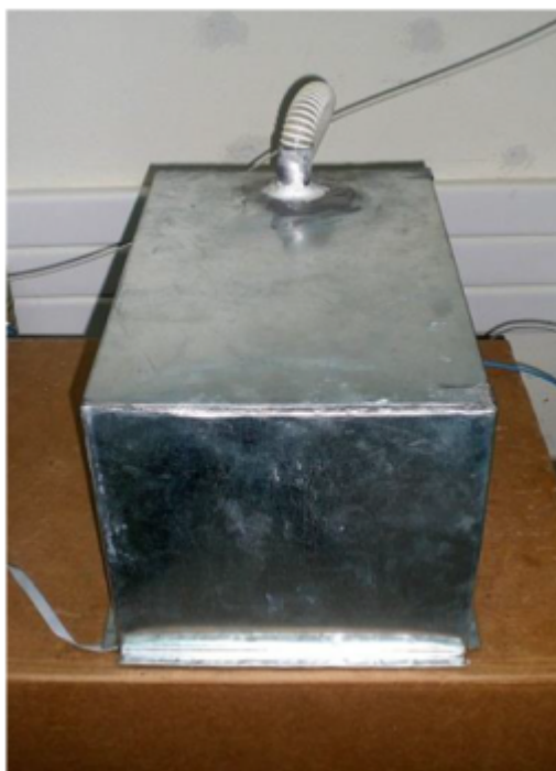
Figure 4.10. Metallic enclosure where the gas measurement cell and mass-flow meters were placed. The enclosure functions as a Faraday cage to avoid electromagnetic interference from external sources. This both protects the sensitive equipment against harmful EMI and provides signal integrity.
