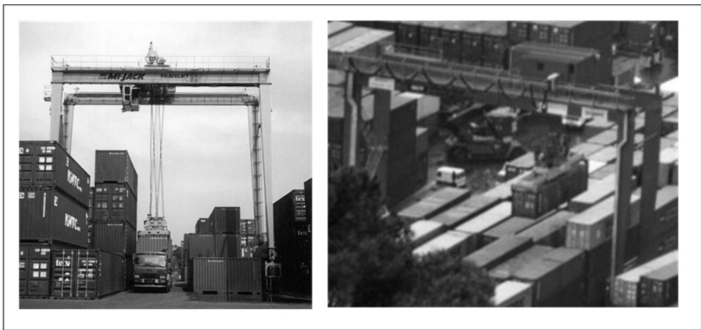
Fig. B.7. Rubber Tyred Cranes at operation
