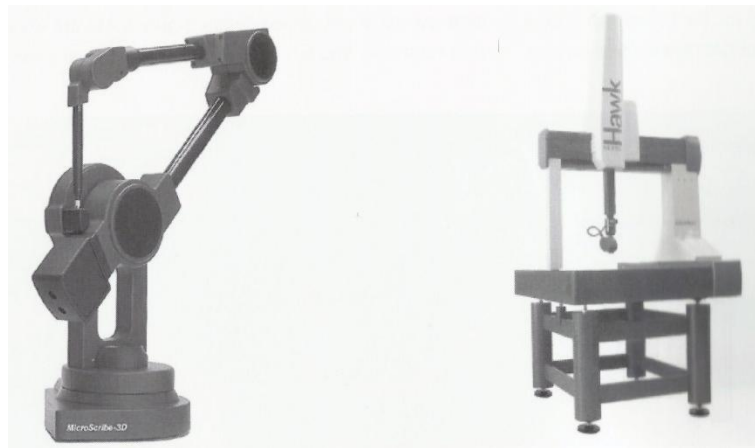
Figure 2. 18. Three dimensional digitizing arm and three dimensional laser scanning machines (Source: Kolarevic, 2009)
