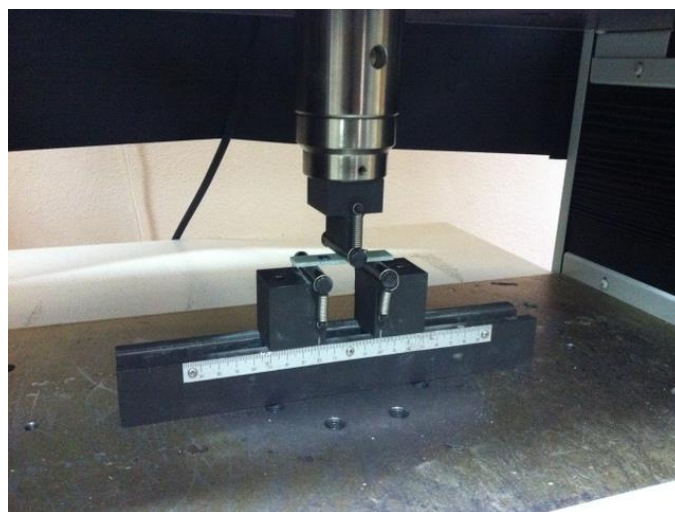
Figure 3.8. Photo of experimental setup for flexural tests
