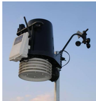
Figure 4.1. Cabled Vantage Pro2™ DAVIS Plus with Standard Radiation Shield
