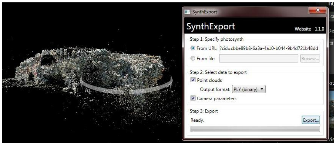
Figure 2.15. Exporting point cloud and camera parameters via SynthExport
