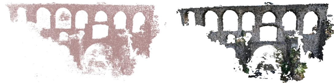
Figure 2.18. Point cloud and mesh construction, Paradiso Aqueduct
