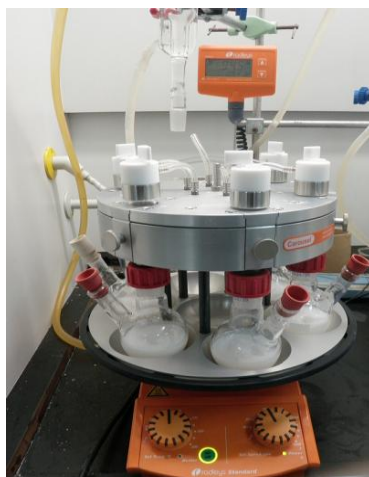
Figure 3.2. Synthesis of AgCl nanoparticles by using carousel multiple synthesis system, The color of the dispersion of AgCl nanoparticles was white.
