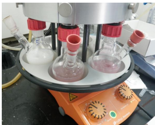
Figure 3.18. Synthesis of AgCl nanoparticles changing the concentration of HCl.
