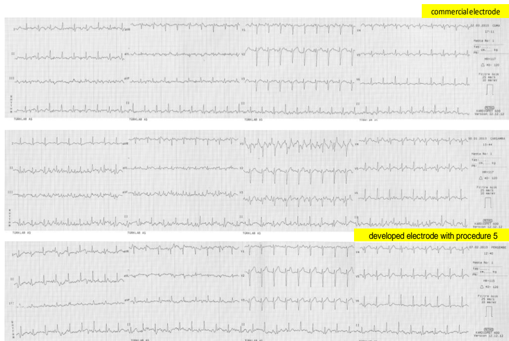
Figure 4.17. Comparative ECG signals observed from the commercial and the new electrodes for cardiac stress test.
