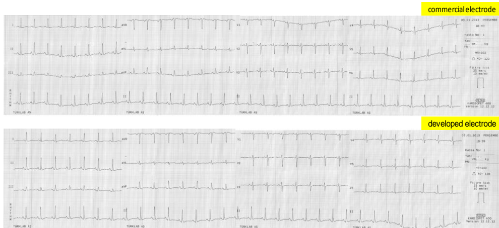
Figure 4.12. Comparative ECG signals observed from the commercial and the new electrodes for cardiac test in motionless patient (Patient A). This new electrode was in the case-4.
