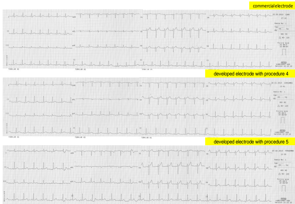
Figure 4.16. Comparative ECG signals observed from the commercial and the new electrodes for cardiac test.
