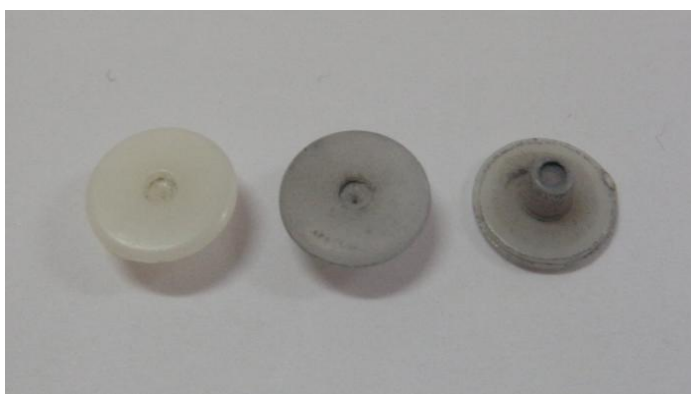
Figure 4.3. Coating of the ABS with the AgCl nanocubes
