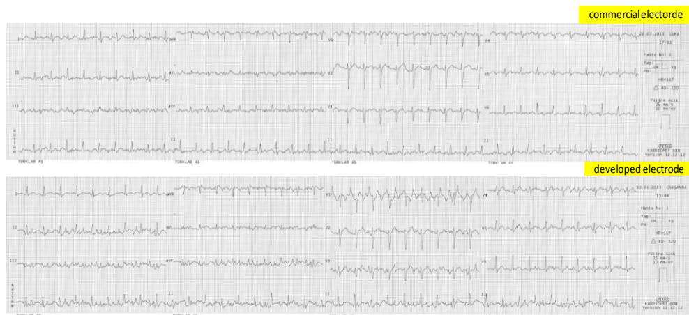
Figure 4.15. Comparative ECG signals observed from the commercial and the new electrode for cardiac stress test (Patient B). This new electrode was in the case-4.
