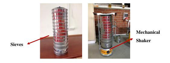
(a) (b) Figure 6.1. (a) Ranged the Sieves #4 to #230, (b) Sieves Column were Placed on the Mechanical Shaker
