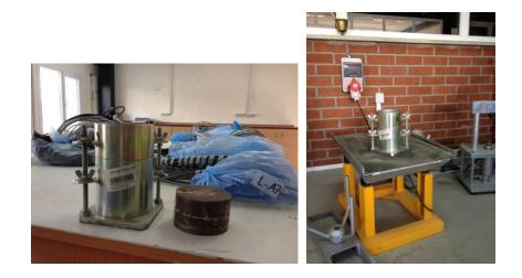
(a) (b) Figure 6.4. (a) Mold and Weight, (b) The Mold Attached to the Vibrating Table
