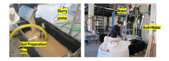
Figure 6.7. Hydraulic Filling Process
