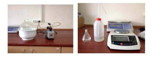
Figure 6.3. (a) Desiccator and Vacuum Pump, (b) Pycnometer, Distilled Water and Weight (Left to Right)
