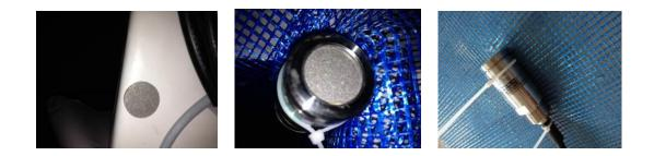
(a) (b) (c) Figure 4.8. (a) Filter of the Pore Pressure Transducer, (b) Filter was Placed inside the Pore Pressure Transducer, (c) Pore Pressure Transducer Used in the Shaking Table Tests
