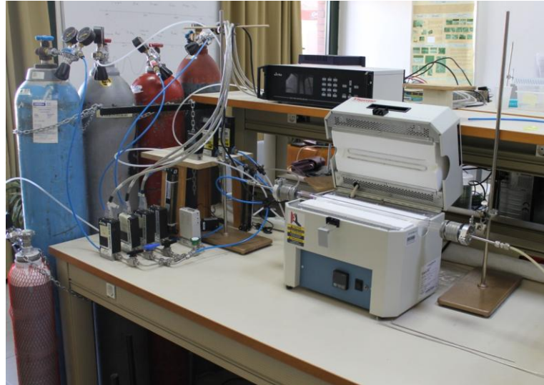
Figure 3.6. CVD growth system at Physics Department, CNL Lab, IZTECH
