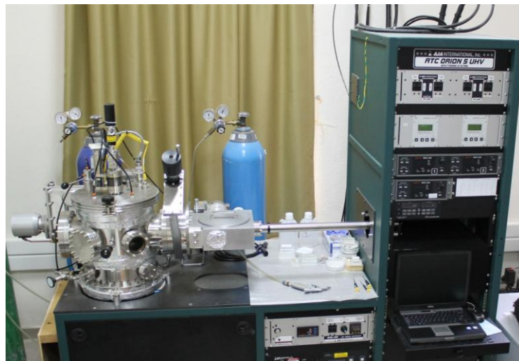
Figure 3.1. ATC AJA Orion 5 UHV Sputtering System in the Department of Physics at IZTECH.
