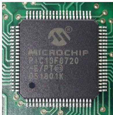
Figure 2.26. A PIC 18F8720 microcontroller in an 80-pin TQFP package (Source: Wikipedia 2012)
