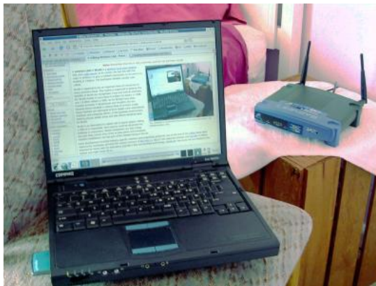
Figure 2.29. A wireless access point connected with a notebook computer through a wireless PC card (Source: Wikipedia 2012)
