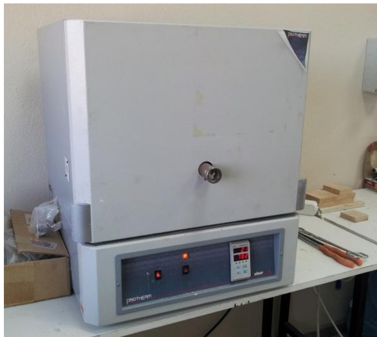
Figure 4.8. Box furnace used in heat treatment.
