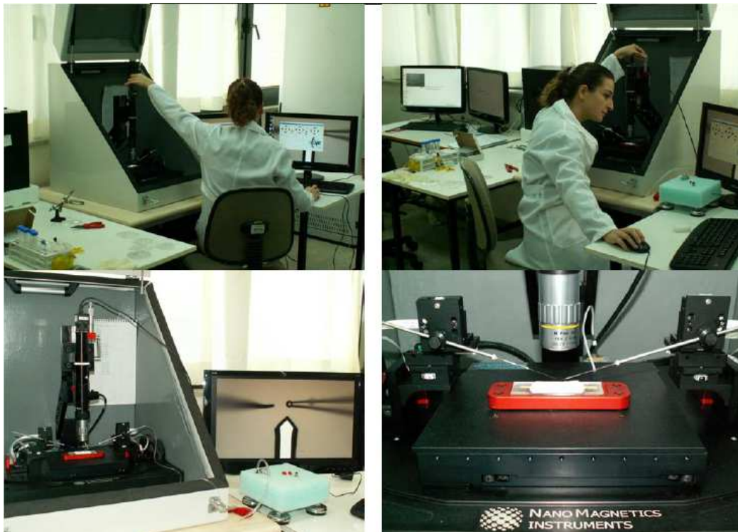
Figure 3.12. Nanomanipulator used to make colloidal probes
