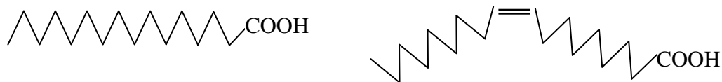
Figure 2.1. The presence of the cis double bond in oleic acid lowers the melting point by 66°C.
