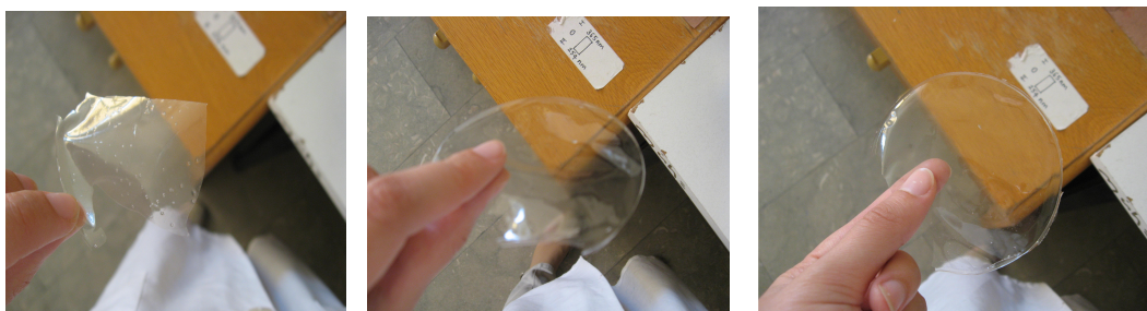
Figure D. 3. Picture of SF film in formic acid (a) Rt loaded SF film (b) IC loaded SF film (c)
