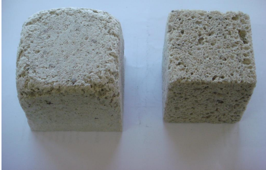
Figure 3.8. The foamed glass before (on the left) and after cutting (on the right).
