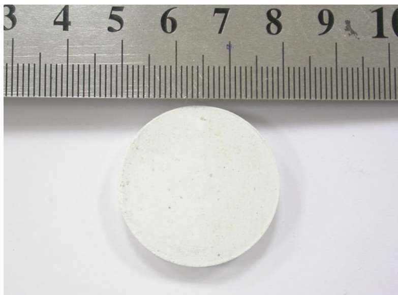
Figure 3.3. The picture of a glass powder compact for expansion experiments.
