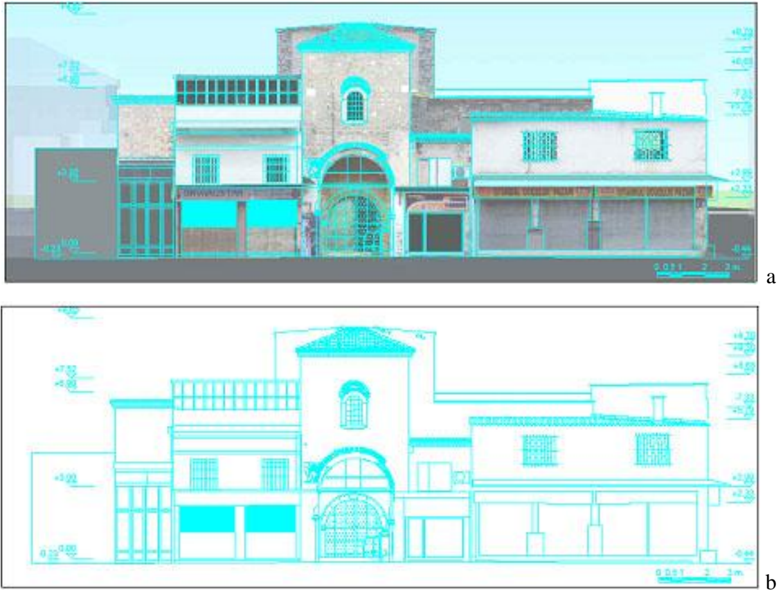
Figure 61. Çakaloğlu Khan, southeastern facade, image from model overlapped with measured drawing (a) Çakaloğlu Khan, southeastern facade, measured drawing (b) (Source: IZTECH, Department of Architectural Restoration - Digital Archive)
