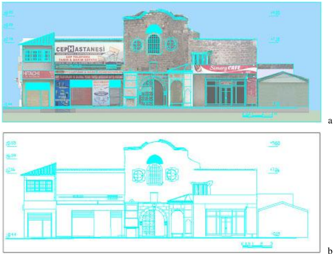
Figure 60. Çakaloğlu Khan, northwestern facade, image from model overlapped with measured drawing (a) Çakaloğlu Khan, northwestern facade, measured drawing (b) (Source: IZTECH, Department of Architectural Restoration - Digital Archive)
