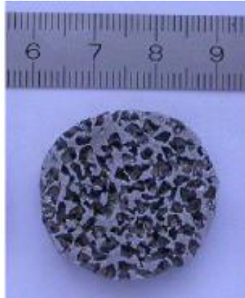
Figure 3.9. Lead foam prepared by the infiltration method, 2 mm in average pore size and 69% porous [31].
