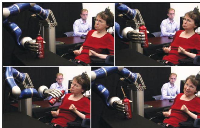
Figure 1.4. Paralyzed woman drinking from a bottle using the DLR Lightweight Robot. (Source: Leigh et al. 2012)
