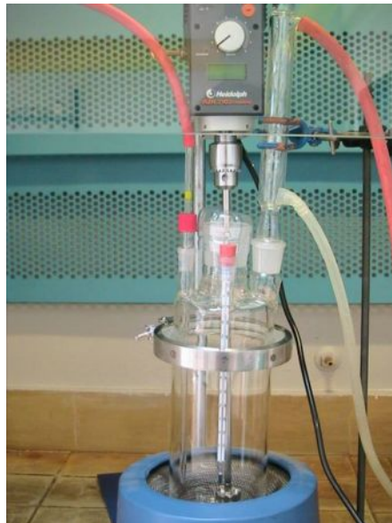
Figure 2.2. Five necked reaction flask used in the synthesis of polystyrene nanoparticles
