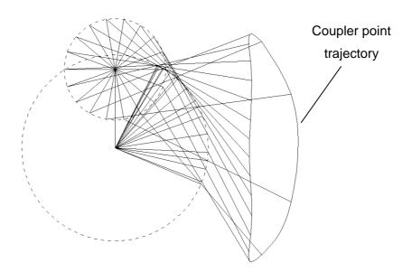
Figure 4-11: Trajectory of one wheel at different positions
