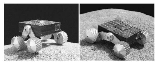
Figure 1-7: Nanorover with active suspension (Courtesy of NASA/JPL-Caltech)
