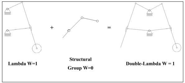
Figure 4-8: Structural synthesis of double-lambda
