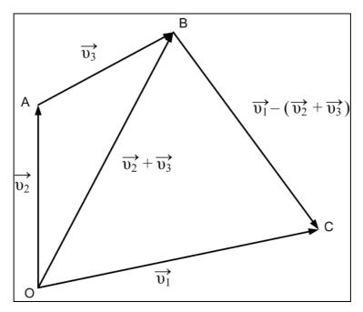
Figure 5-2: Vector loops on lambda mechanism
