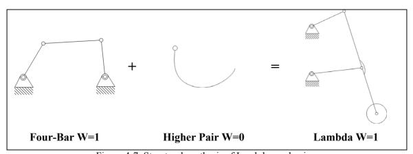
Figure 4-7: Structural synthesis of Lambda mechanism
