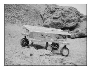
Figure 1-8: Micro5 rover with suspension named Pegasus (Courtesy of Meiji University – Japan)
