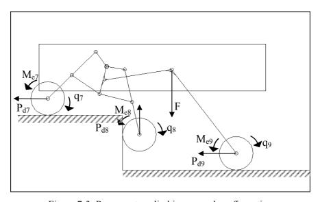
Figure 7-3: Reverse step climbing second configuration
