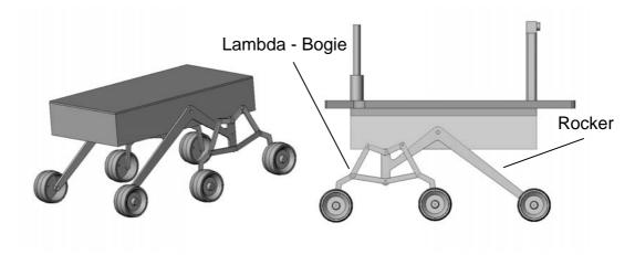
Figure 4-15: Experimental suspension design LBS
