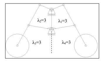
Figure 4-1: Kinematic diagram and closed loops of bogie mechanism
