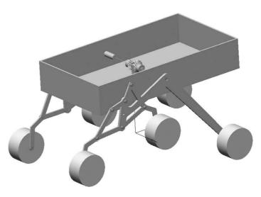
Figure 8-1: Rover computer model for simulation
