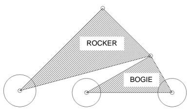
Figure 2-5: Kinematic diagram of Rocker-Bogie suspension
