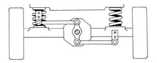
Figure 3-1: Watt's linkage application on rear-suspension
