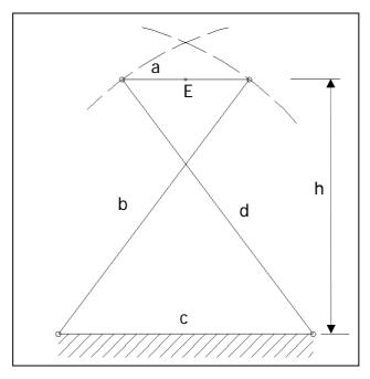
Figure 3-2: Cross-link straight line mechanism by Chebyshev
