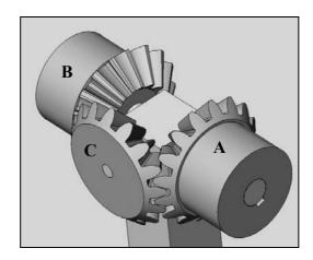
Figure 4-16: Differential gear mechanism between right and left rockers
