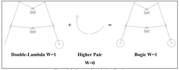
Figure 4-9: Structural synthesis of bogie
