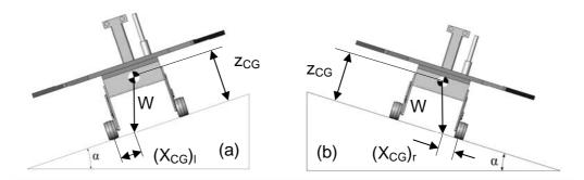
Figure 6-4: Lateral stability margins and dimensions
