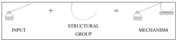
Figure 4-3: Structural synthesis with one input and one structural group
