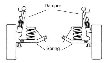
Figure 2-1: Independent car suspension system with damper and spring
