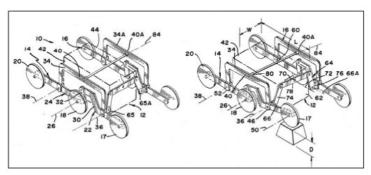
Figure 2-4: Articulated Suspension System (US 4,840,394)
