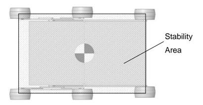
Figure 6-2: Stability area consists of contact points
