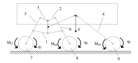
Figure 7-1: Equivalent forces and virtual displacements of LBS
