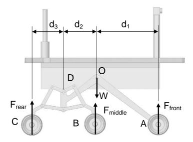
Figure 6-1: Force diagram of LBS
