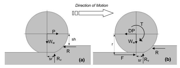
Figure 2-3: Free body diagrams of towed (a) and driven (b) wheels [26]
