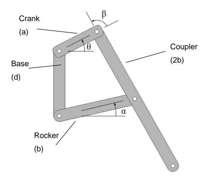
Figure 4-10: Definition of linkages and crank angle
