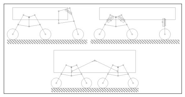
Figure 4-18: Different applications of lambda bogie suspension
