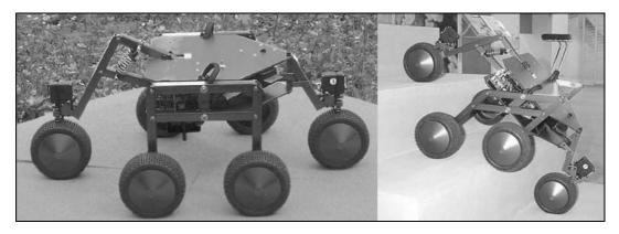
Figure 1-9: Shrimp rover designed by EPFL – Switzerland (Courtesy of EPFL)
