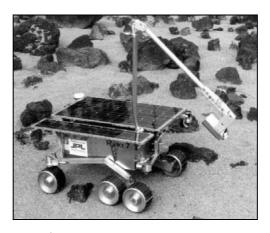
Figure 1-5: Rocky 7 Rover (Courtesy of NASA/JPL-Caltech)
