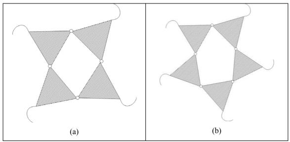
Figure 4-5: Closed kinematic chains with 4 (a) and 5 (b) structural groups
