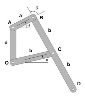
Figure 5-5: Transmission angle
