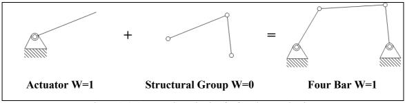
Figure 4-6: Structural synthesis of a four-bar mechanism
