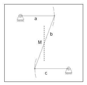
Figure 3-3: Watt's Approximate Straight-Line Mechanism
