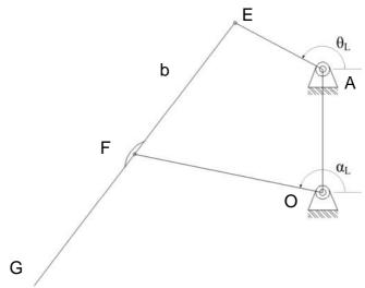
Figure 5-6: Left side of the bogie mechanism
