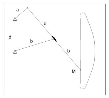
Figure 3-5: Lambda Mechanism
