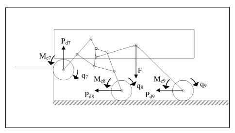
Figure 7-2: Reverse step climbing first configuration
