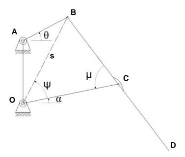
Figure 5-3: Angles between linkages
