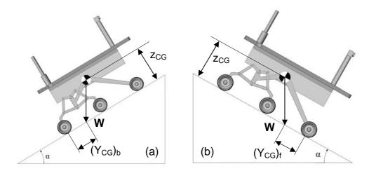
Figure 6-3: Downhill rear (a) and front (b) stability margins and dimensions
