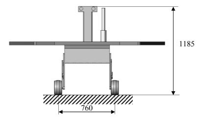
Figure A1.1: General dimensions of the rover (Front View)
