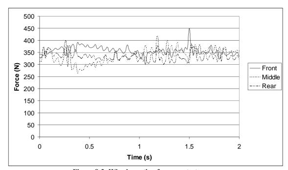
Figure 8-3: Wheel reaction forces on test course
