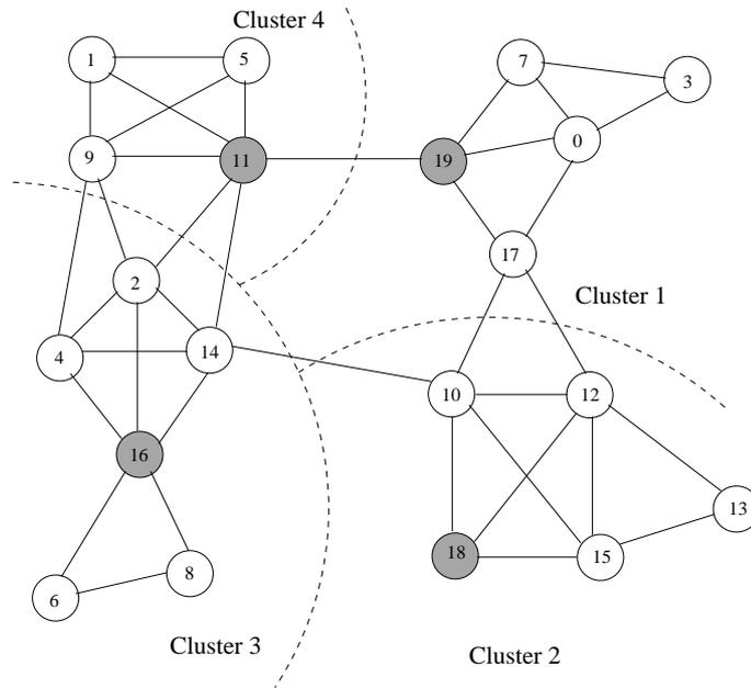
Figure 3.3. Clusters obtained using Merging Clustering Algorithm
