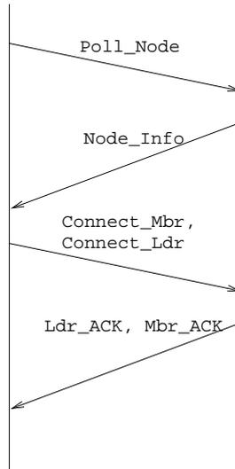
Figure 3.2. Message Flow Diagram of Merging Clustering Algorithm
