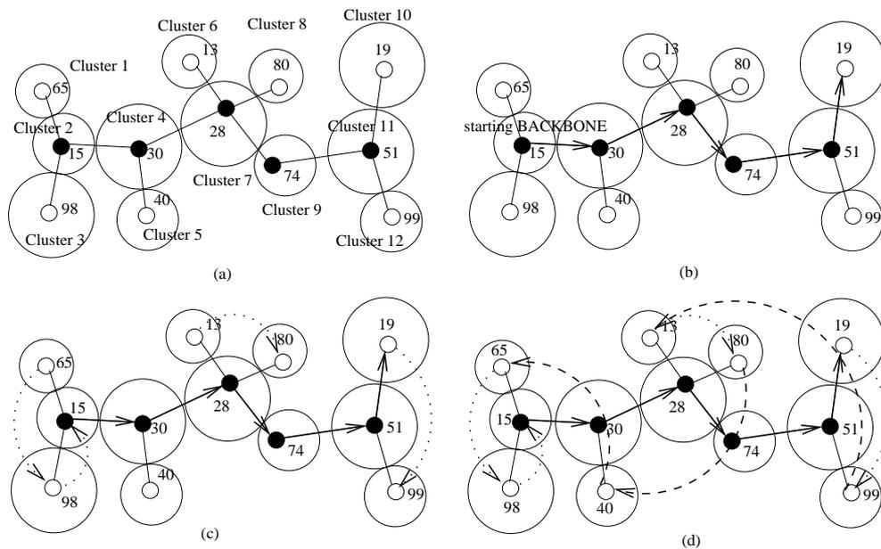
Figure 4.3. An Example Operation for Backbone Formation Algorithm
