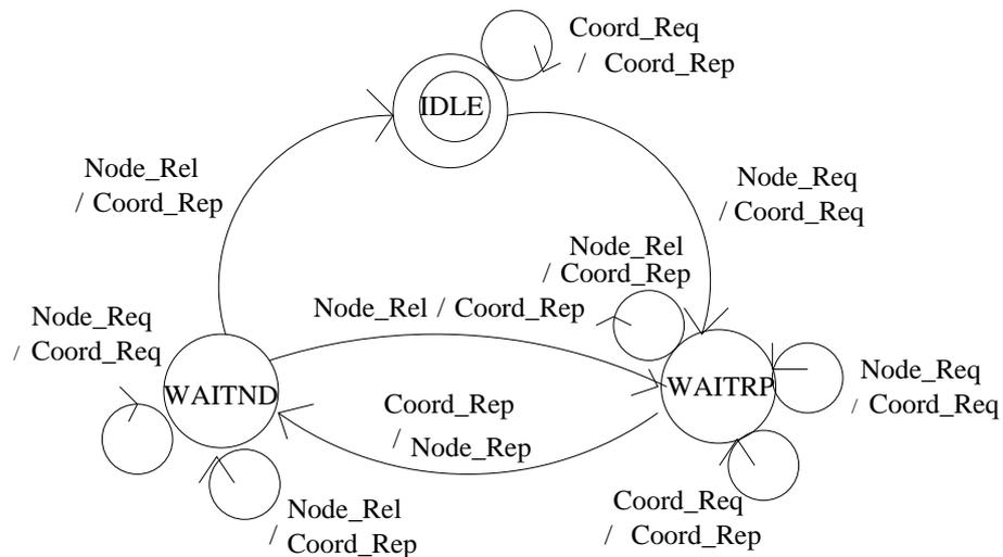
Figure 5.1. Finite State Machine of the Mobile\_RA Coordinator
