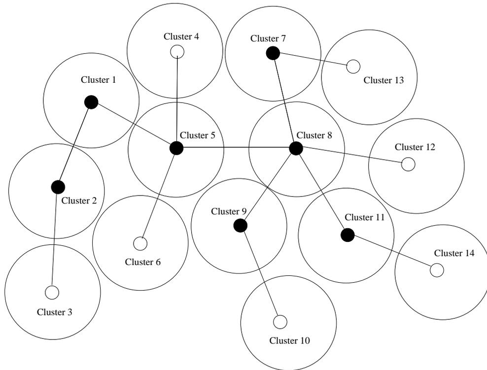
Figure 4.2. A MANET with its minimum spanning tree
