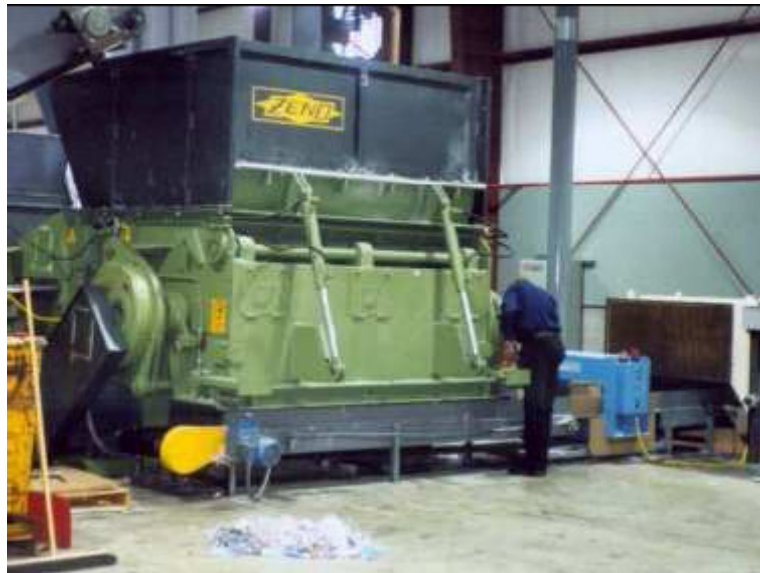
Figure 5.20 A single shaft rotary shredder
