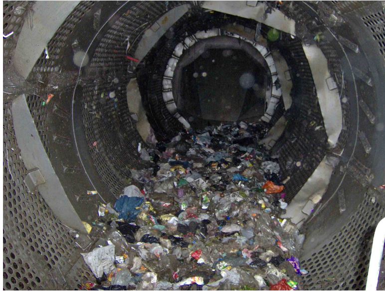
Figure 3.9 Inside of the trommel that has 45 mm diameters of holes
