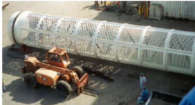
Figure 5.5 a trommel prior to installation
