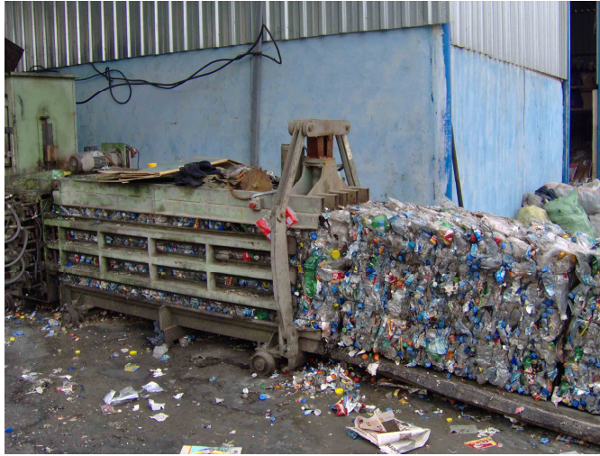
Figure 5.19 A baler and its package
