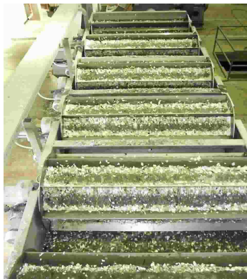
Figure 5.13 Rotating part of the float tank
