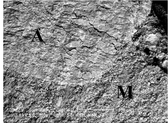
Figure 4.68 Detailed BSE image (500×) of the left-handed image, showing how well the aggregate (A) was adhered to the mortar matrix (M).
