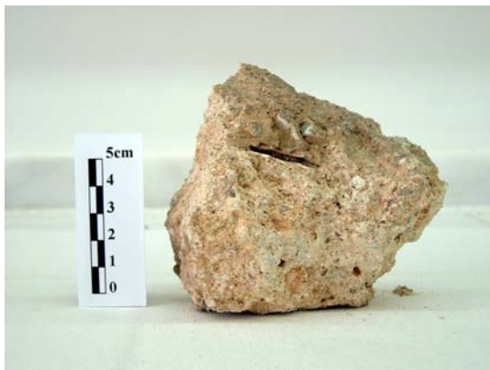
Figure 3.5 Stone masonry mortar sample (Se.Dü.s.) taken from the Düzce Bath.
