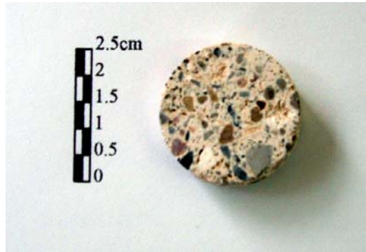
Figure 3.20 Cylindrical specimen drilled from the mortar sample of Se.Dü.b.
