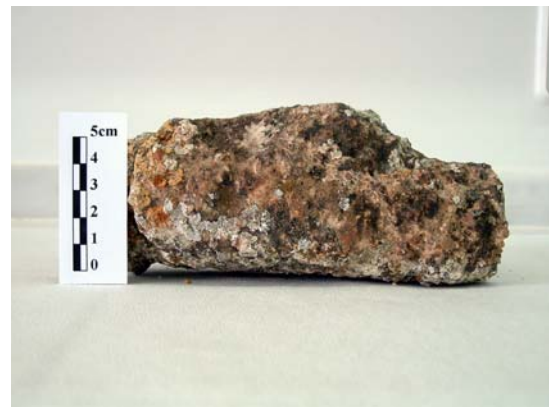
Figure 3.6 Brick masonry mortar sample (Se.Dü.b.) taken from the Düzce Bath.
