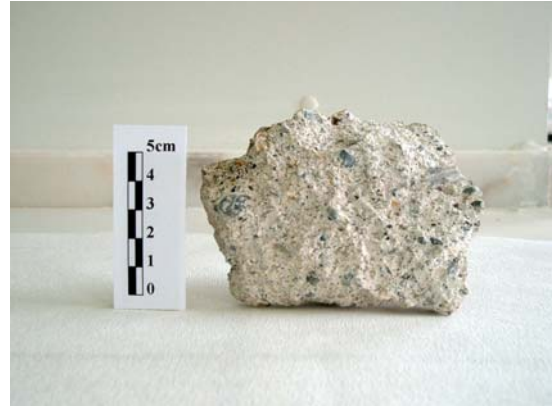
Figure 3.11 Brick masonry mortar sample (Se.Ul.b.) taken from the Ulamiş Bath.
