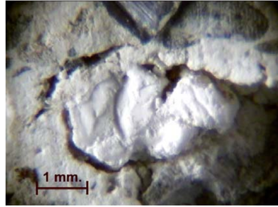
Figure 4.21 Stereo microscope image of the white lump in the stone masonry mortar sample of Se.Ul.s.
