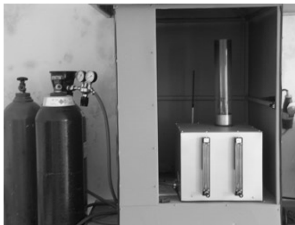
Figure 3.7: Apparatus of limiting oxygen index test.
