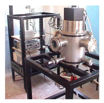
Figure 3.8. (a) Schematic representation of Ar-ion beam system (b) the photograph of the same system.
