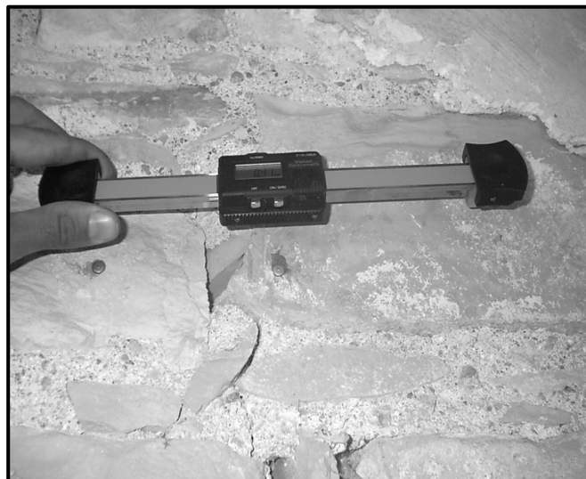
Figure 4.12. Crack measuring device
