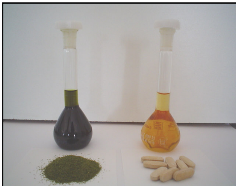
Figure 3.1: Extracts of Ginkgo leaf powder and the commercial GNC tablets obtained by solvent extraction.
