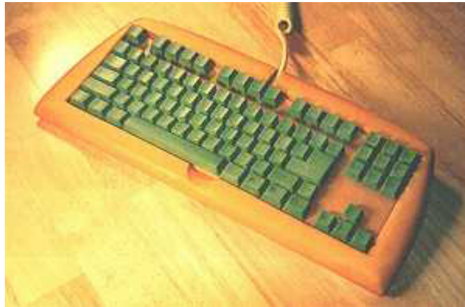
Figure 3. 14. ‘The Compostable Keyboard’ computer keyboard made of carrot pulp, keys of spinach and celery.
