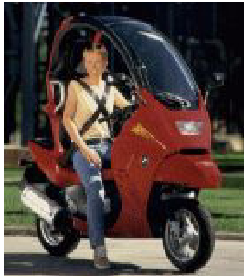
Figure 2. 14. BMW R1 roofed scooter makes it easier for people to get onto two wheels..no helmet required
