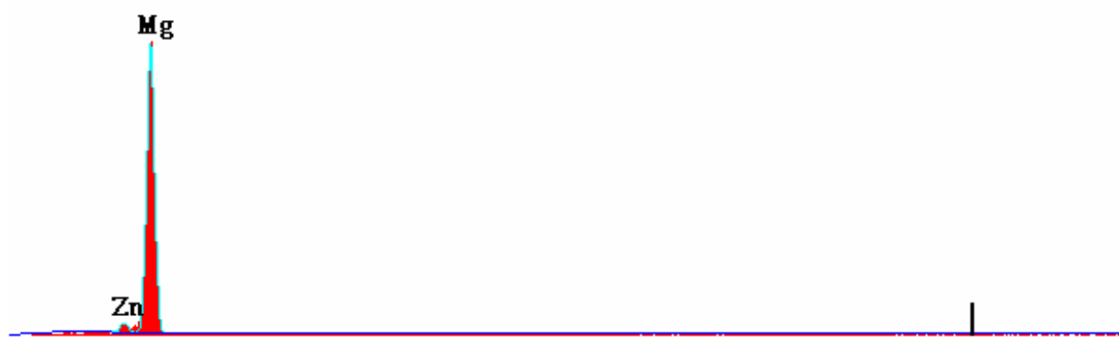
Figure 5.1 EDAX analysis of Mg grains.
