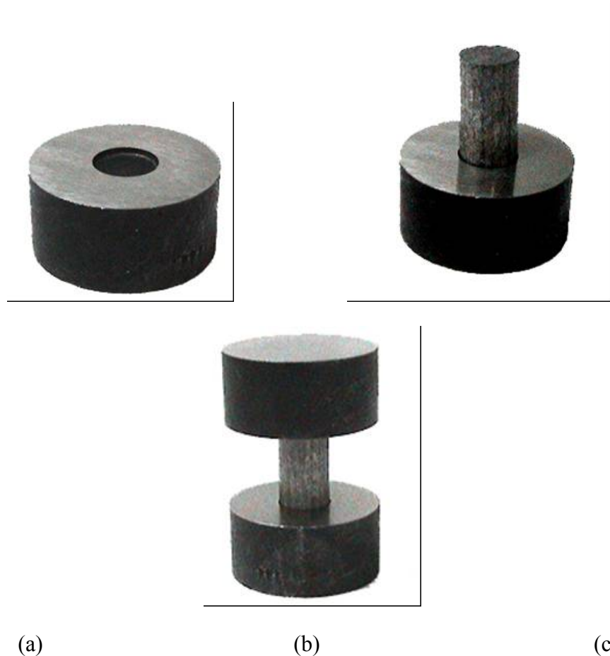
Figure 4.4 a) Steel tap used in axial tests ,b and c) insertion of test samples into the steel caps
