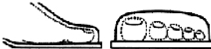
Figure. 4.57. The space allowance for a foot in any footwear design
