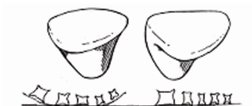
Figure. 3.68. Left, concave-bottom last (common) causing “falling” of middle metatarsal heads; right, flat bottom last (rare) allowing normal flat plane of metatarsal heads.
