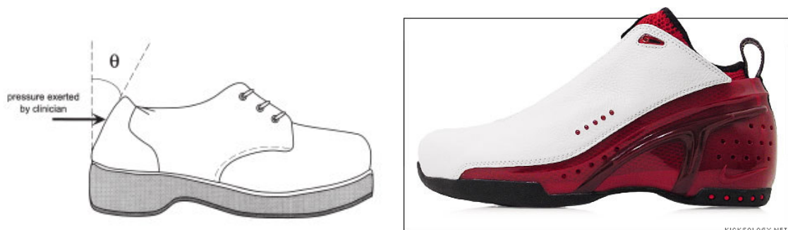
Figure. 4.54. Assessments of heel counter stiffness and an example from NIKE
