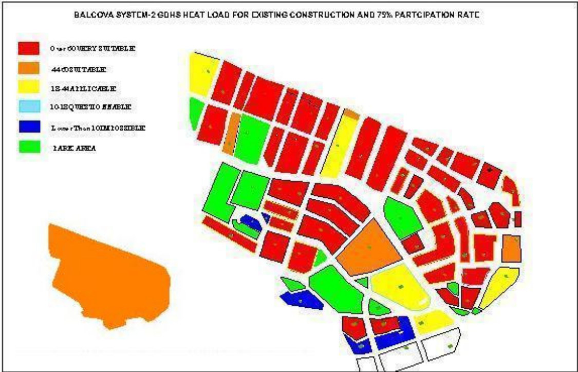
Figure 4.3b. Heat load density distribution for existing buildings and 75% participation rate.
