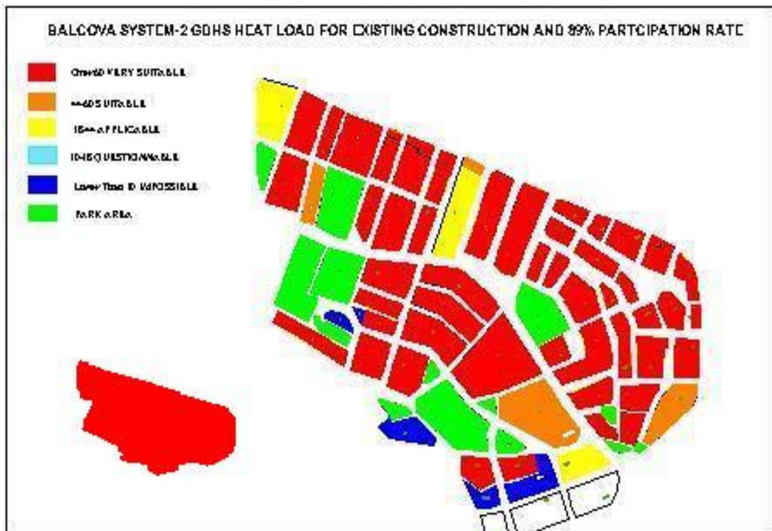
Figure 4.3a. Heat load density distribution for existing buildings and 89% participation rate.
