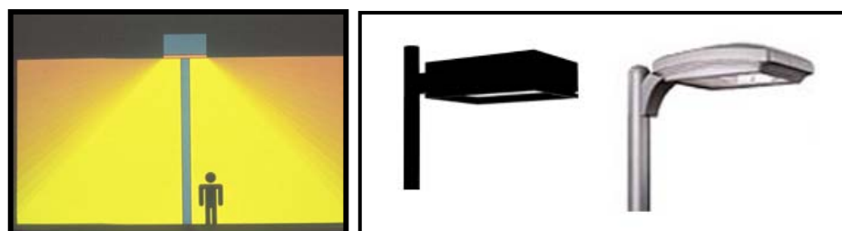
Figure 2.11. Cut-off luminaires (Source: IDA, http:// www.darksky.org )
