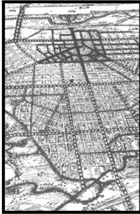
Figure 3.8. Lighting zones by category of street in a hypothetical city. (Source: Harrison et.al. 1930, p.22)
