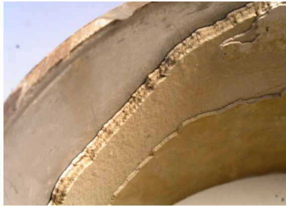
Figure 1.8. Stainless steel pipe scaling layer section
