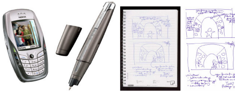
Figure 4.31. Elements of the iDeas notebook. Left to right: camera phone; digital pen; physical notebook page after Idea Log activities; electronic file automatically created from notebook page.
