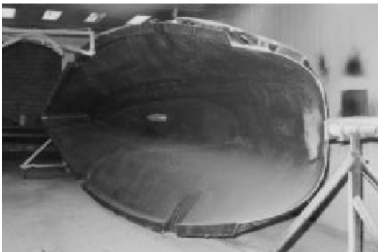
Figure 4.5. Production Female Mold on Spindle at Corsair Marine (Greene 2004)
