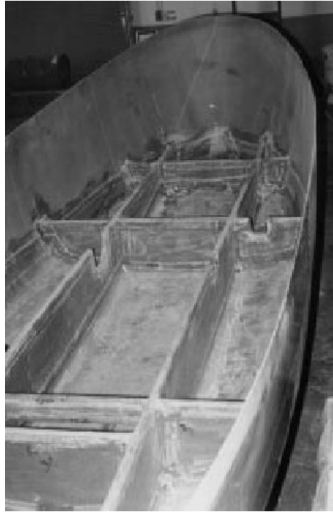
Figure 4.34. SCRIMP U.S. Coast Guard Motor Lifeboat Built by OTECH. (Greene 2004)
