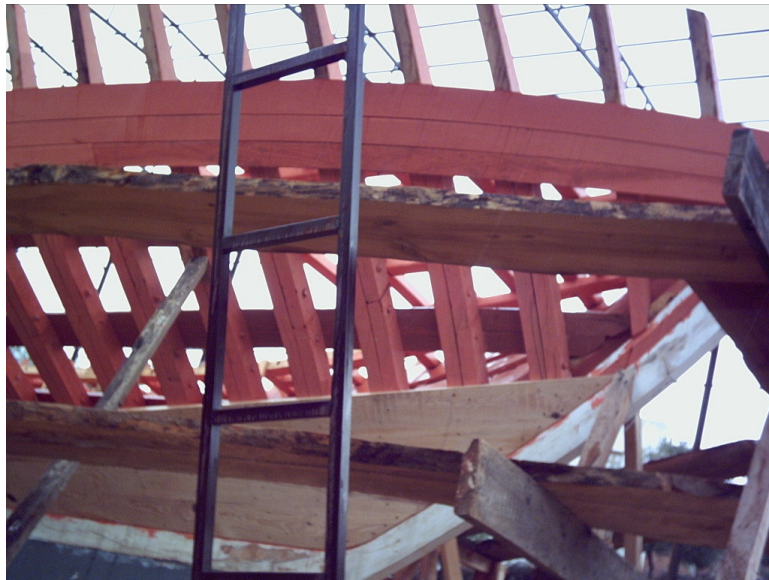
Figure 4.57. Wooden Framework of a Gulet. (Gölpınar 2004)
