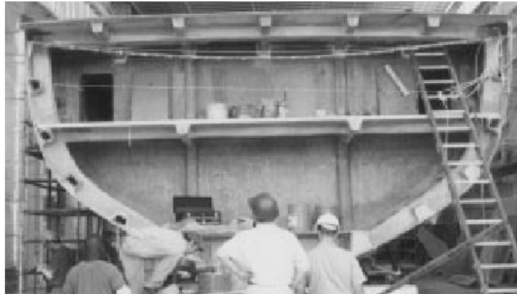
Figure 4.47. One-Half Scale Corvette Hull Test Section Built for the U.S. Navy Using the Sunrez Process (Greene 2004)
