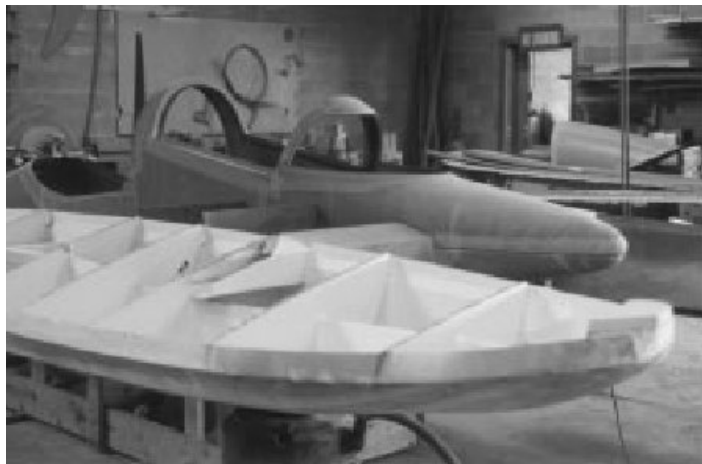
Figure 4.41. Hydroplane Hull and Cockpit Assemblies at Ron Jones Marine (Greene 2004)
