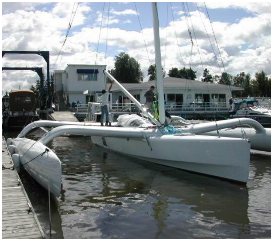
Figure 2.1. Antrim 40' Racer / Cruiser Trimaran-hull: Composite sandwich construction with Kevlar and carbon fiber reinforcements. WEB_1 (2004)
