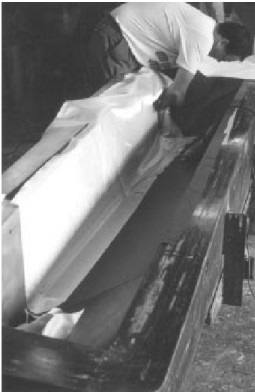
Figure 4.38. Prepreg Material is positioned in Mold (Greene 2004)
