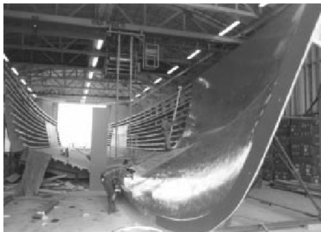
Figure 4.7. Batten Construction of Female Mold at Westport Shipyard (Greene 2004)
