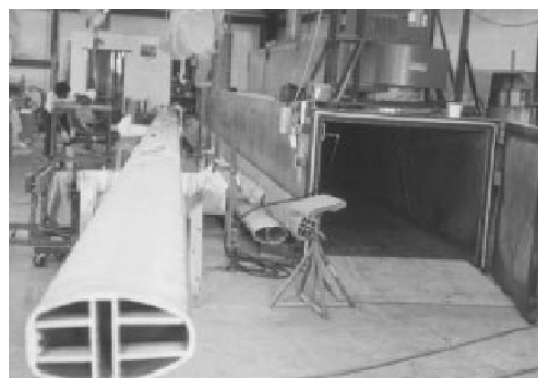
Figure 4.42. Cure Oven Used for Masts and Hardware at Goetz Marine Technology (Greene 2004)
