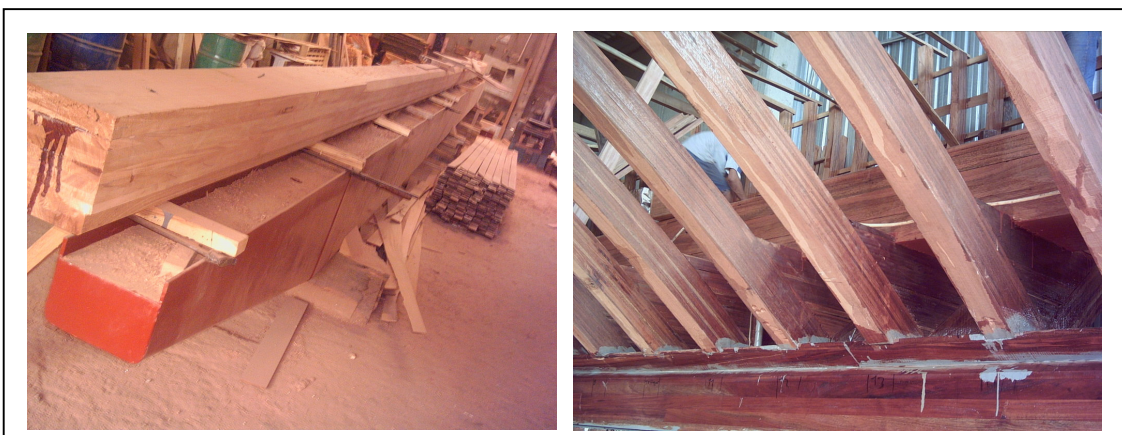
Figure 4.59. Laminated ballast and keels. (Gölpınar 2004)
