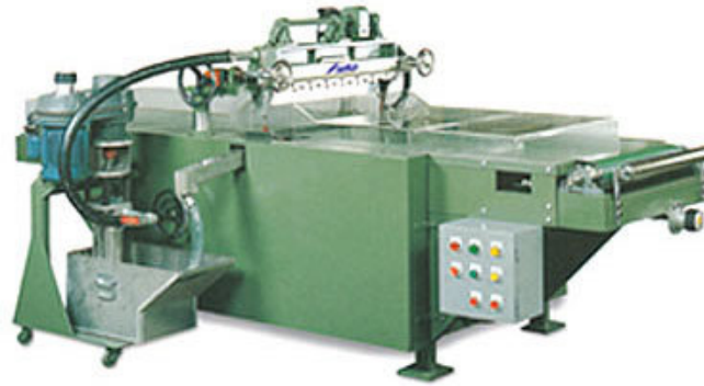
Figure 4.9. Flow coater WEB_18 (2004)
