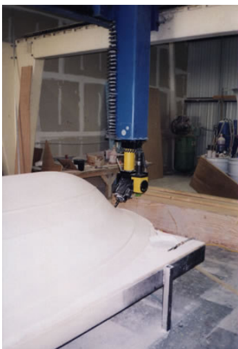
Figure 4.50. CNC milling for hull WEB_19 (2004)
