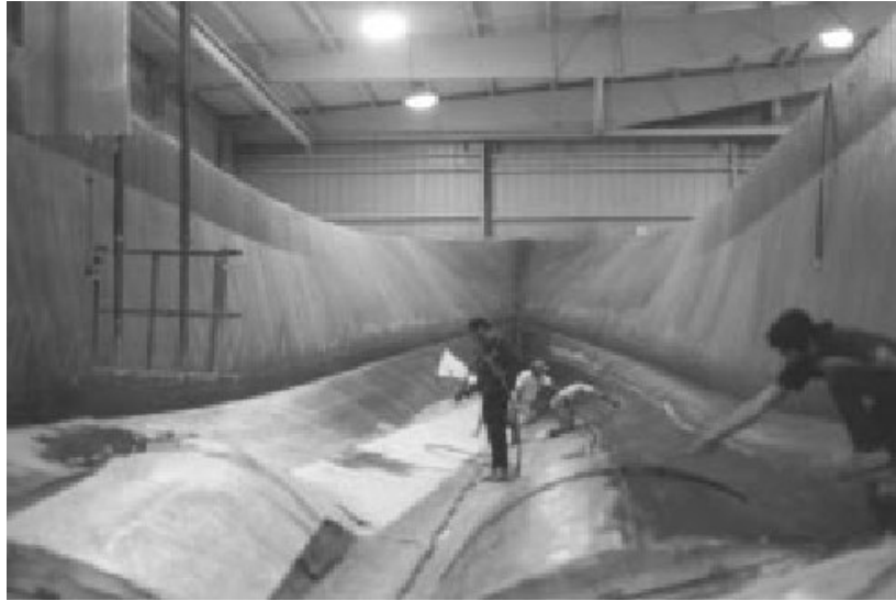
Figure 4.18. Laminators Consolidate Reinforcement Material Applied by Impregnator at Westport Shipyard. (Greene 2004)
