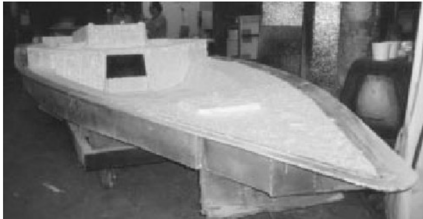
Figure 4.32. Dry Reinforcement In-Place for SCRIMP Process (Greene 2004)
