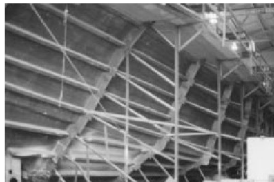
Figure 4.6. Metal Stiffened Female Mold at North coast Yachts (Greene 2004)
