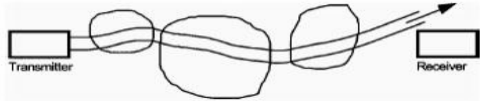
Figure 2.15. Laser beam wander due to the turbulent cells that are larger than beam diameter.
