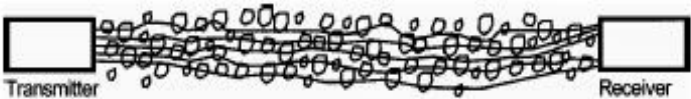
Figure 2.14. Scintillation in beam intensity due to the turbulent cells that are smaller than beam diameter.
